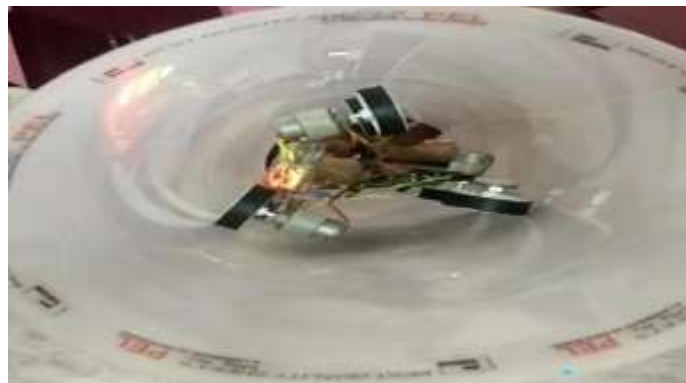
Fig 16 Picture showing working of PIR inside the pipe
